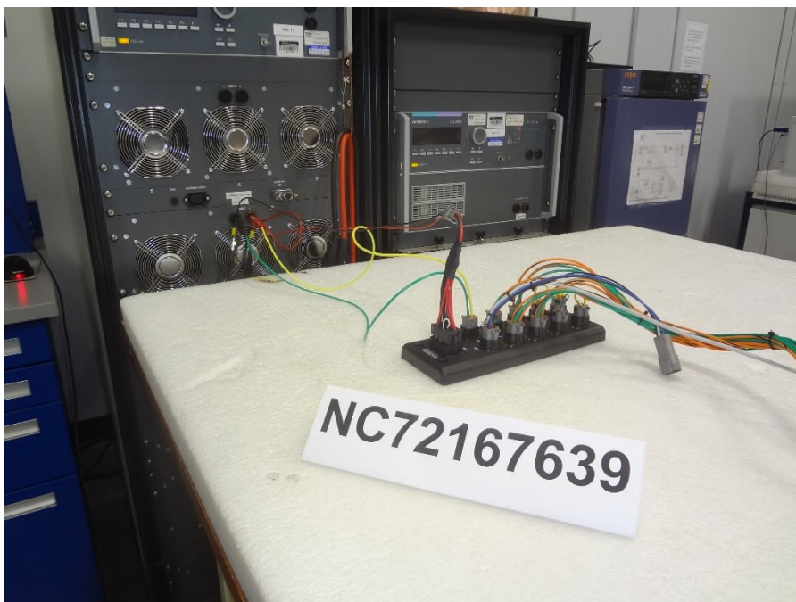
Photo 2.4-2 – Immunity to Conducted Transients on Power Leads – Pulses 2b and 4
