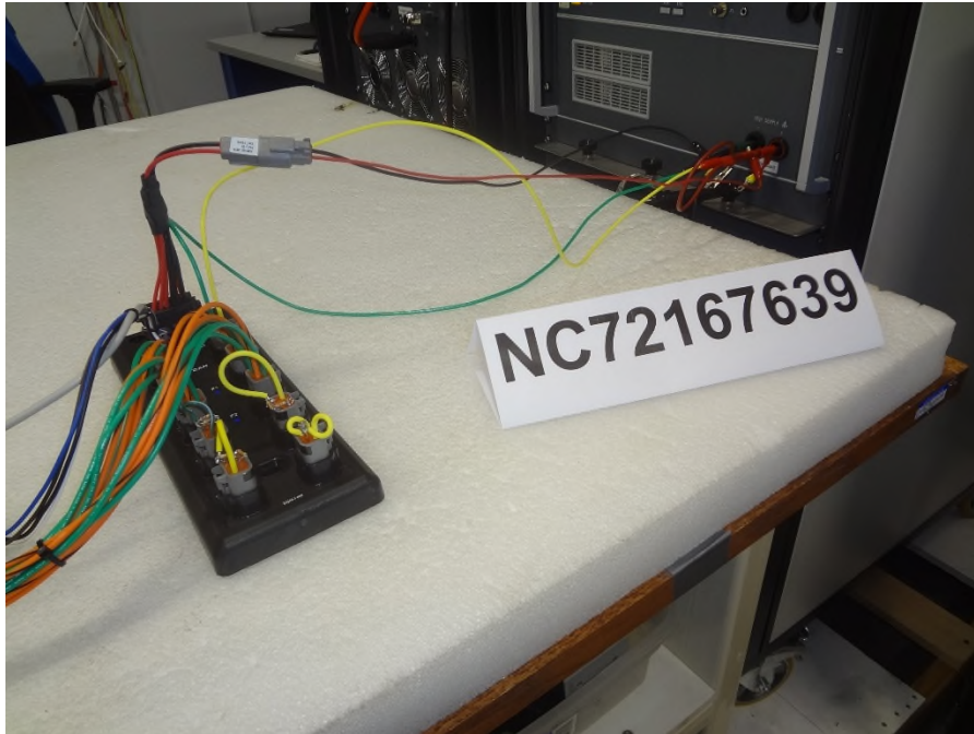
Photo 2.4-1 – Immunity to Conducted Transients on Power Leads – Pulses 1, 2a, 3a, and 3b
